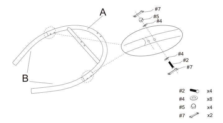
Step 2. Attach plastic clips (part #6) to assembled unit (parts A & B).
